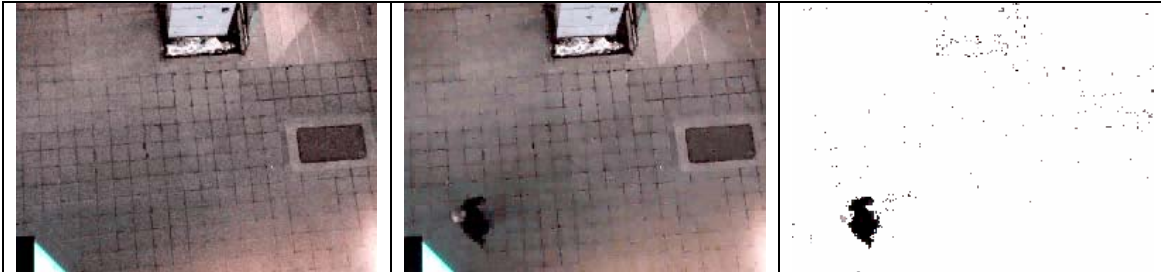
Figure 4. Background image (left), one slice in an image sequence (middle), result of subtracted images (right)
