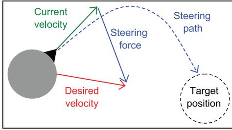
**Figure 1.** The steering force produced by the Seek behavior is the vector difference between the agent's desired velocity (the vector pointing from the agent to the target position) and its current velocity, as given by Helbing et al.<sup>2</sup>
