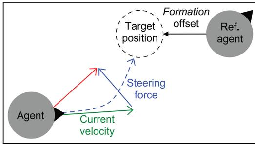
**Figure 3.** The steering force produced by the *Formation* behavior is a *Seek* steering force directed toward the position of a specific reference agent with an added offset.
