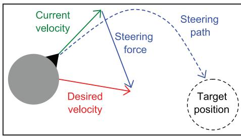
**Figure 1.** The steering force produced by the *Seek* behavior is the vector difference between the agent's desired velocity (the vector pointing from the agent to the target position) and its current velocity, as given by Helbing et al.<sup>2</sup>
